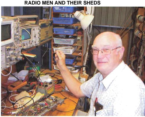
materials and assorted adaptors. Above on the equipment shelf are two oscilloscopes, a Hewlett Packard signal generator, power supplies and a home-built signal tracer unit. To the right of the bench is a large stand holding dozens of reels of wire and cable. Nearby is a Traeger 'flying doctor' transceiver and shelves containing dozens of neatly labelled plastic bins of components.
