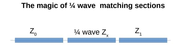
Suppose we want to match an antenna that has A feed point impedance of 300 Ohms to 50 Ohm Coax The ¼ wave matching section impedance can be calculated As follows, mutiply the input and output impedances together and take the square root, that's the impedance of the matching quarter wave section.
