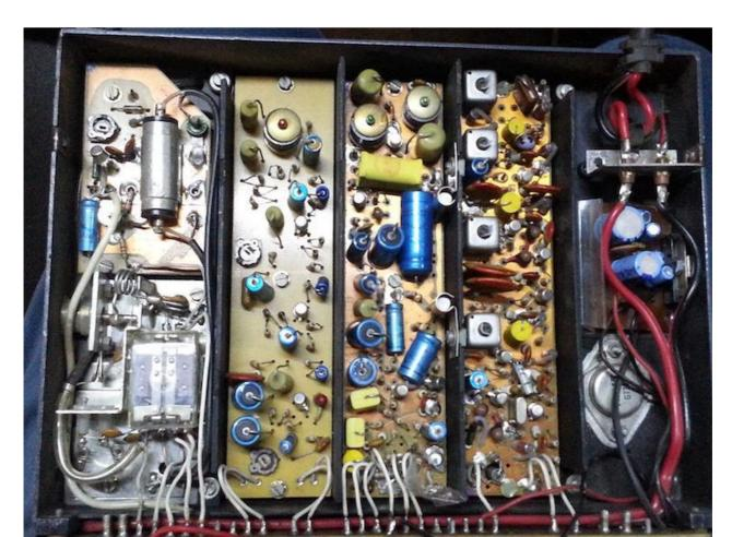
My aim is to replace the RX oscillator/multiplier board with a custom PCB that has the Arduino Nano, Si5351 and CTCSS R2R DAC.
