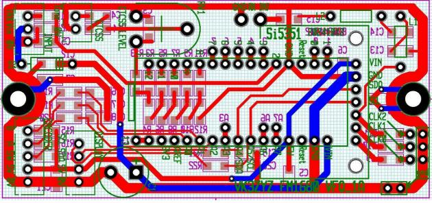
This PCB design is similar to my "normal" Arduino Nano VFO but with a few refinements to add RF stoppers on the external leads as the prototype using my original VFO board would crash as the power was tuned up on TX.
