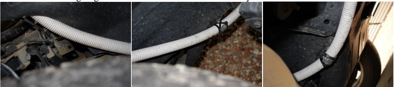
Route of DC cable going to underside of vehicle between body and wheel arch.
