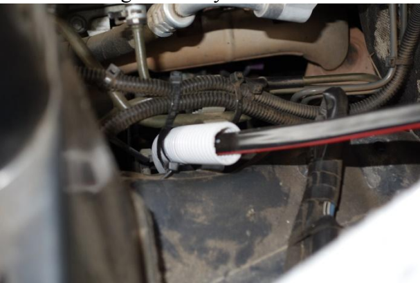
Route of DC cable going to underside of vehicle between body and wheel arch.
