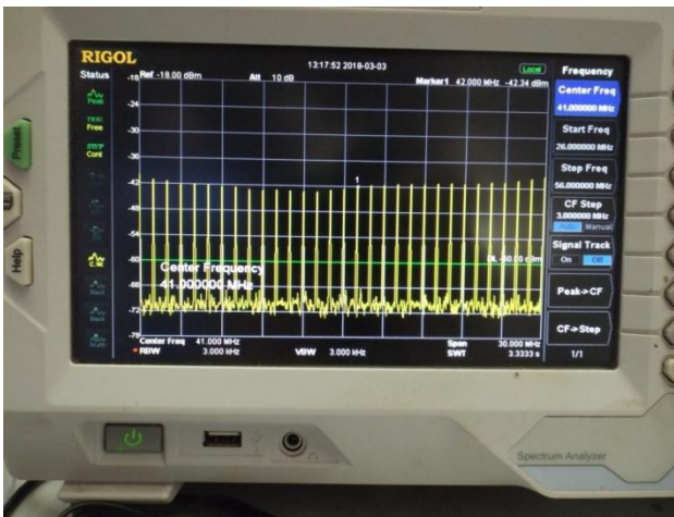
The output of Bill's comb generator shown on the spectrum analyser.
