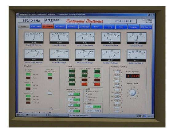
This is the control/indicator panel for the Continental 418G AM/DRM 100 kilowatt transmitter at Radio Australia. Sadly no longer are the meter readings occurring.
