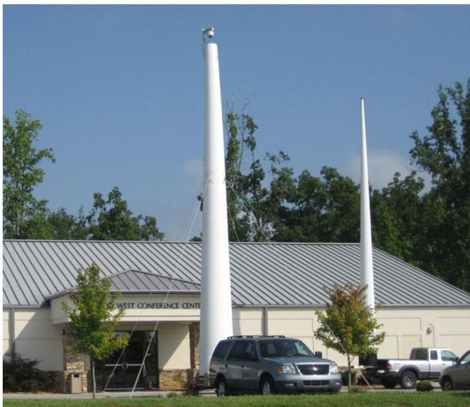
These portable inflatable towers are everything you need to quickly put up your antennas/repeaters, video, or sensor payloads after emergencies or at large public gatherings. They're portable enough to mount on any vehicle so you can enhance your radio or mobile phone range on any remote operation. The COMET version will even put a high quality video camera 37 ft in the air. Our camera can be viewed and controlled from a computer or PDA from anywhere in the world!
