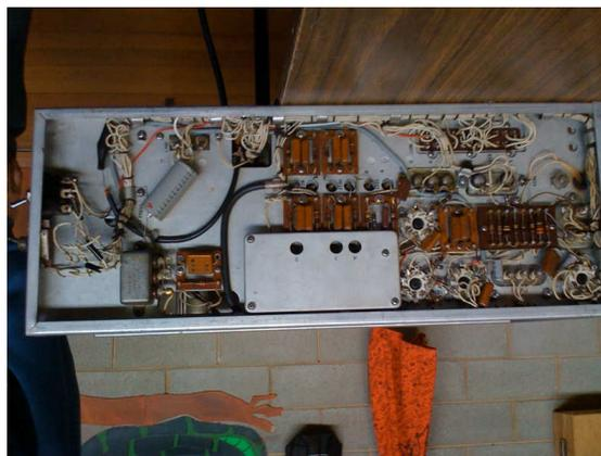
These pictures give some idea of the complexity of the unit. The unit is a 105A/ARR-15 receiver. It was designed for use as an auto tune unit in combination with the autotune ART-13 transmitter. The receiver can be manually tuned if you lock the autotune mechanism and you can also manually tune the transmitter in a similar manner.
