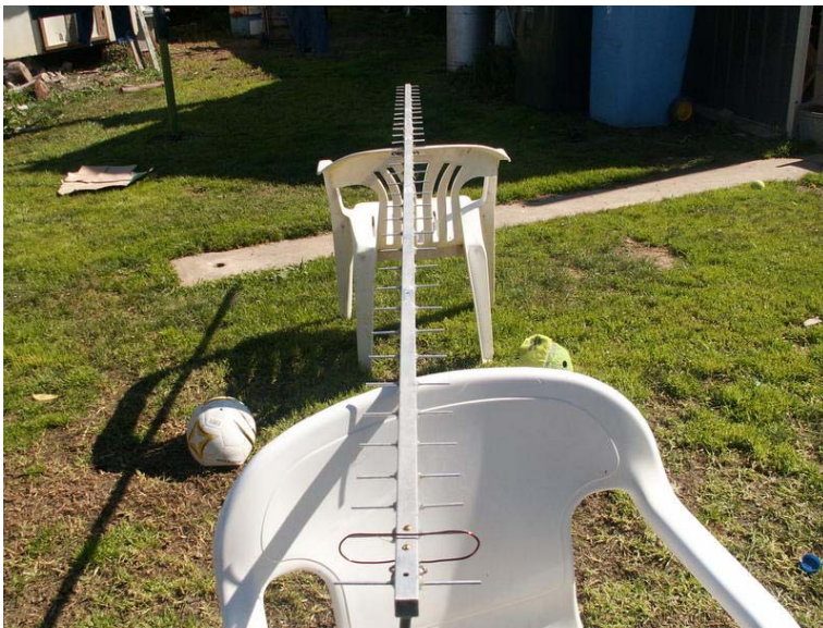
The finished 1296 Mhz 36 element beam. And it works to. Dinki Di!
